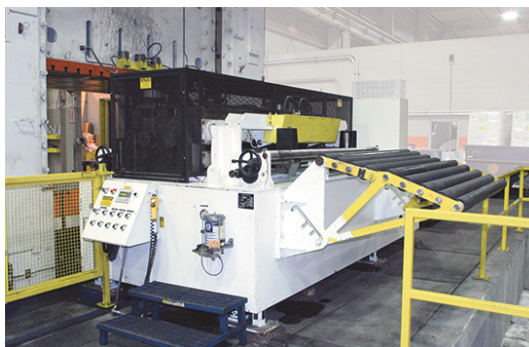
To equip its blanking department to handle 72-in.-wide coils of high-strength steel as thick as 0.400 in. thick, Voss Clark sought a coil feeder that could stand up to the rigorous task at hand. Called to action: a four-roll servo feeder from Cooper-Weymouth Peterson.
