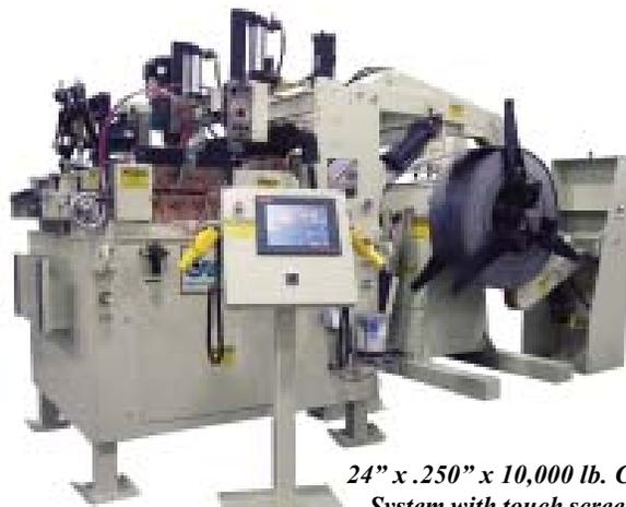
*24" x .250" x 10,000 lb. Compact Coil System with touch screen interface*
