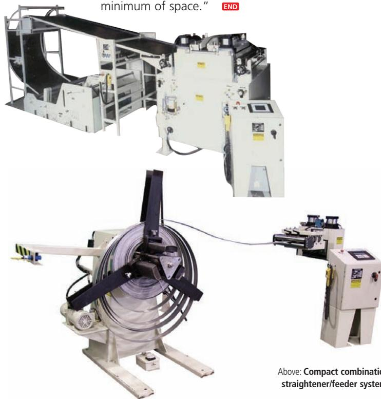
Above: **Compact combination straightener/feeder system.**
