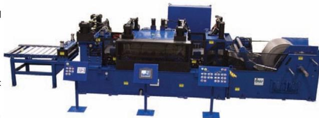
which pay off material from the top through an overhead loop chute arrangement. This design allows for a back load of the coils directly into the cradle section of the system. A heavy duty hydraulic debender unit accepts the lead edge of the coil and breaks it for easy thread-up into the straightener/feeder unit.
